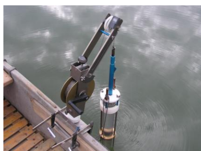
Fig. 1. Sediment sampling device (UWITEC).
